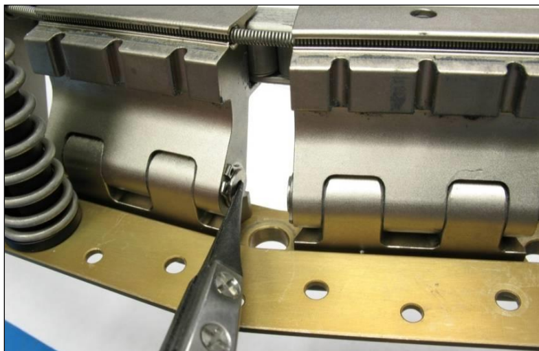
Figure 7-1: Pushing Leaf Pin to side to make room for SHC screw (15.000-24 only).
