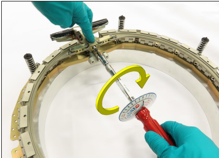
Figure 8-3: Rotating ball screw to allow Sliding Tube travel
