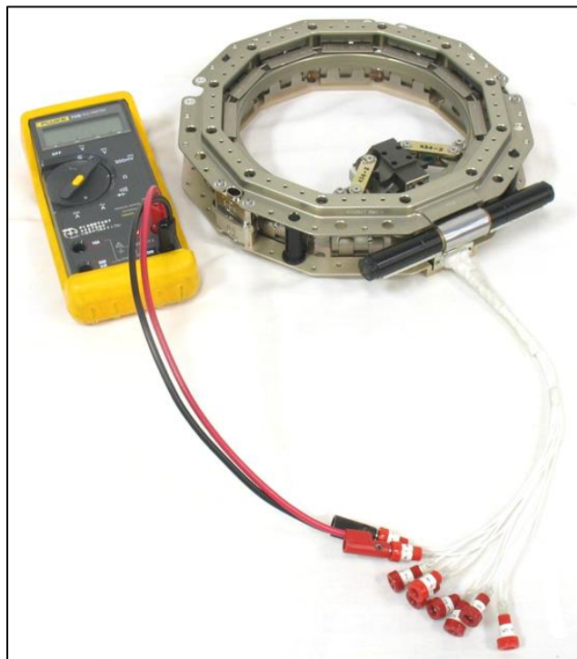
Figure 16-2: DMM and DB-9 breakout cable used to measure Motor Bracket Assembly resistance.
