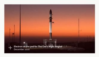
The mission will launch from Rocket Lab Launch Complex 1 on New Zealand's Māhia Peninsula to an initial elliptical orbit, then Electron's Kick Stage will perform a series of burns with its relightable Curie engine to raise apogee and act as a space tug to deliver the OHB Cosmos' payload to its precise orbital destination.
