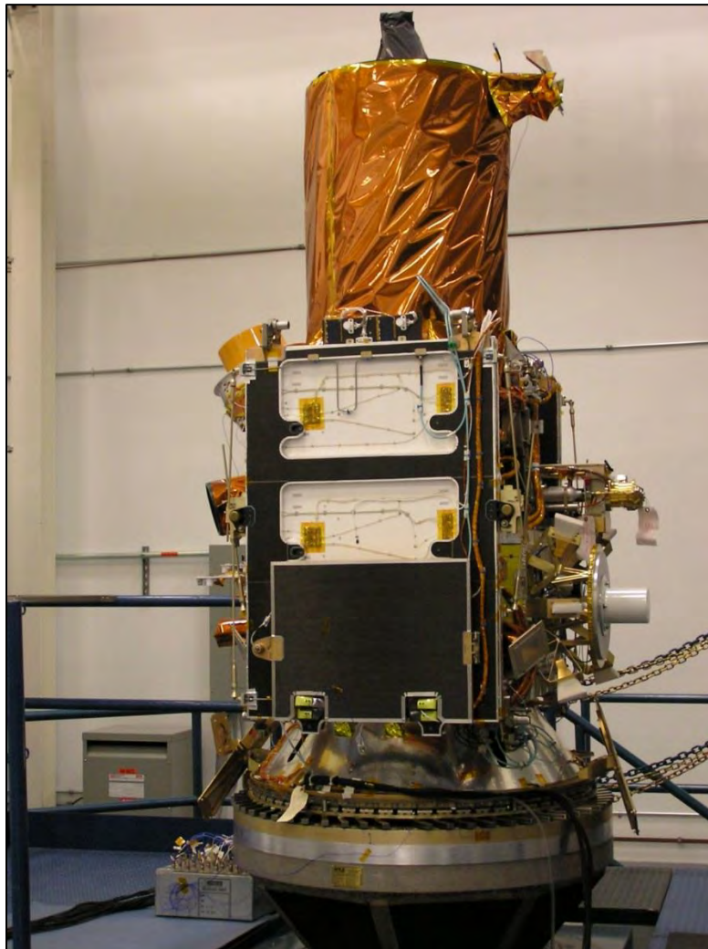
Figure 4-1: An MLB installed on the TacSat-2 mission
