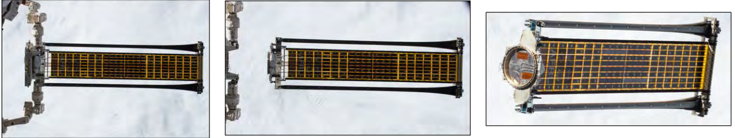
Figure 14-1: 23 inch MLB deploying ROSA from ISS
