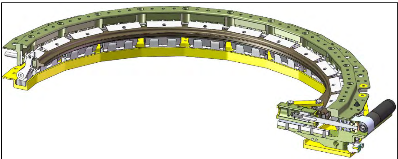
Figure 7-6: The Leaves disengaged during deployment, (section view)
