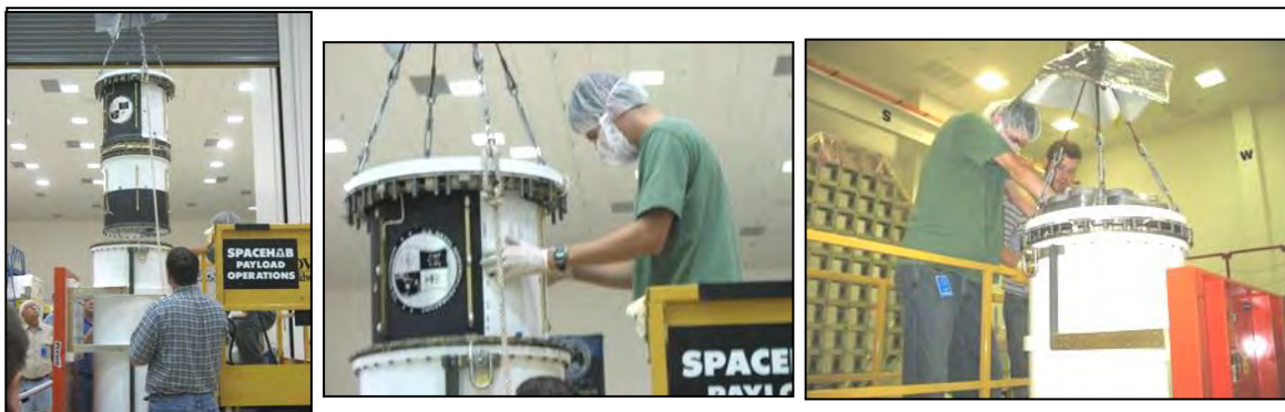
Figure 15-4: PSC engineers perform a vertical integration (CAPE-ICU-I)
